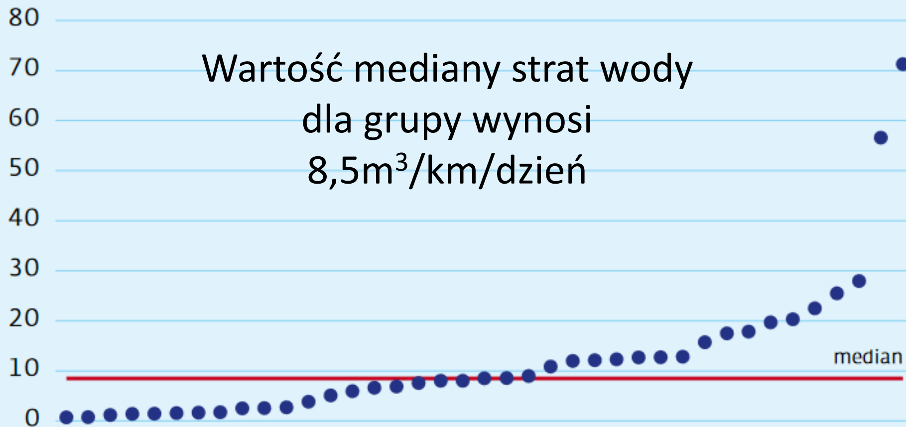
Figure 4: Distribution losses per mains length (m 3 /km/day)
